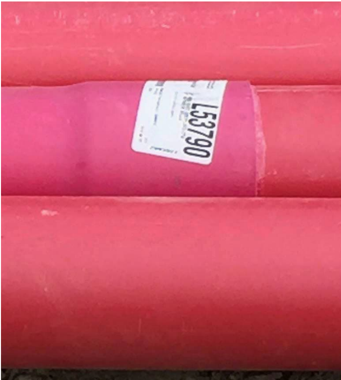
Note white glue residue at the seam
